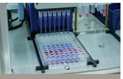
OpenTrons liquid handling robot used for malaria assays.
