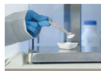
Weighing out of chemical compound for making a solution.
