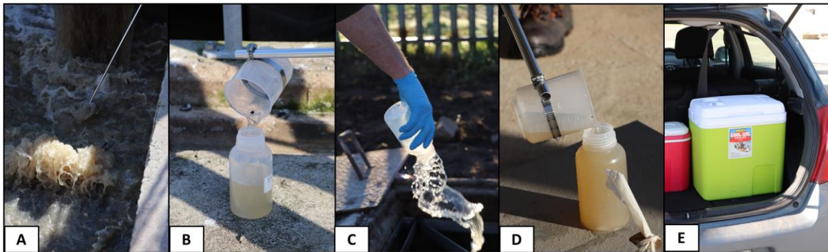
Figure 2: Wastewater grab sampling. A) Collect wastewater with the grab sampling device, after rinsing in the wastewater. B) Pour into the labelled sample bottle, avoid contaminating the outside of the bottle. C) Rinse the inside of the sample bottle with the wastewater and discard of the contents. D) Repeat steps A&B and fill the sample bottle to the brim and close the lid tightly. E) Spray down the sample bottle with 70% ethanol and transport on ice.
